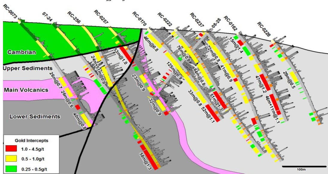
Figure 2: Section 429525E illustrating intercepts and the continuity of the mineralization in the Sunshine Zone.
