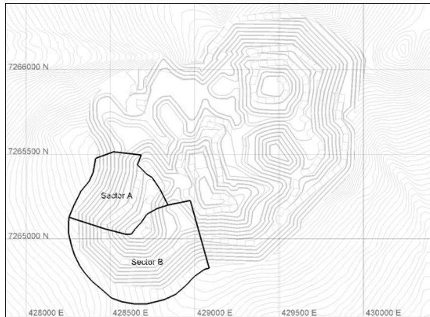
Figure 12-4: Pit Slope Design Sectors for the Ultimate Pit
