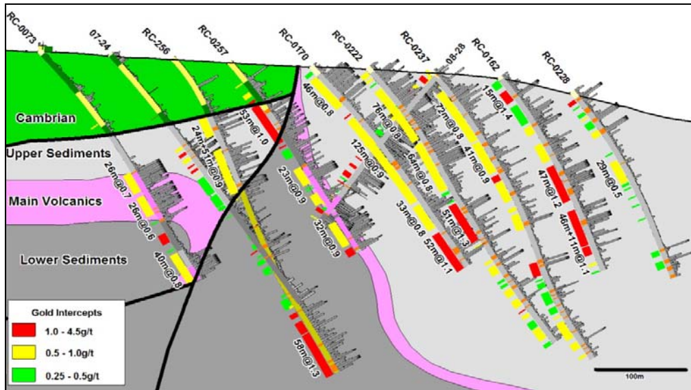
Figure 1: Section 429525E illustrating intercepts and the continuity of the mineralization in the Sunshine Zone.
