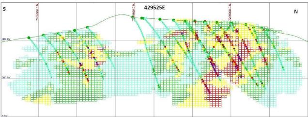
Figure 19.4. Block model for section 429075 E. Grid squares are 200m.
