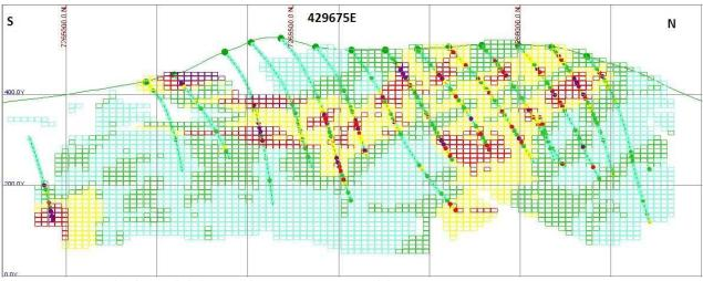
Figure 19.6. Block model for section 429675 E. Grid squares are 200m. 20.0 Recommendations
