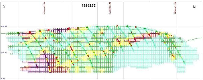
Figure 19.1. Block model for section 428625 E. Grid squares are 200m.
