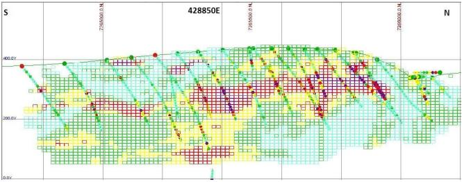
Figure 19.2. Block model for section 428850 E. Grid squares are 200m.
