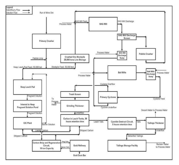
Figure 16.3 Alternate Livengood process block flow diagram showing both heap leach and mill / CIL process streams
