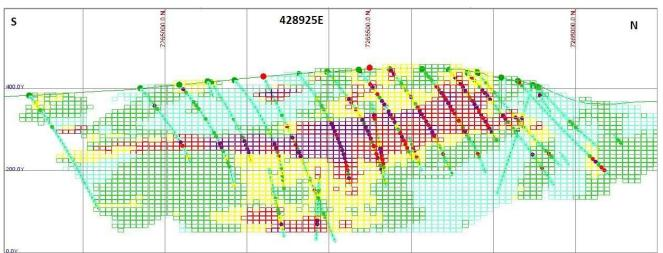
Figure 19.3. Block model for section 428925 E. Grid squares are 200m.
