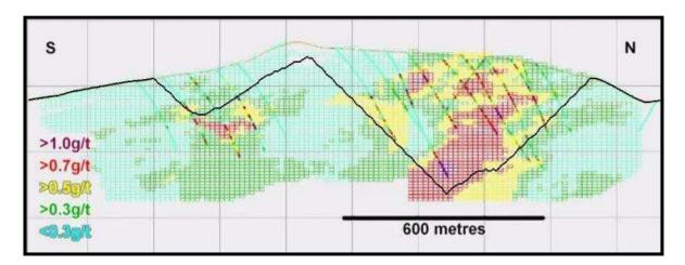
Figure 19.2. Block model for section 429525 E.
