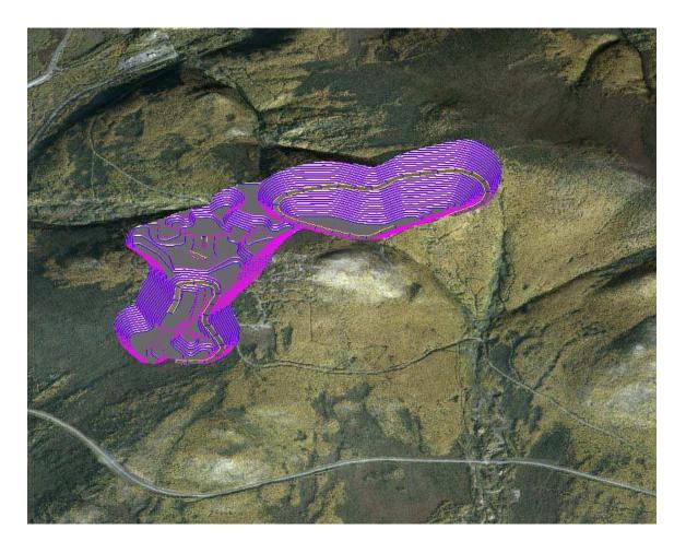
Figure 18-2 Heap Leach Only Pit Design shown in a geo-referenced perspective view of the Money Knob Deposit Location. North is toward the top of the view.
