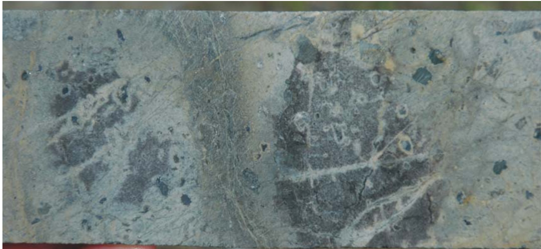
Fig. 3 Remanent patches of potassic (dark) in sericitic alteration (light). MK-08-33, 190 m
