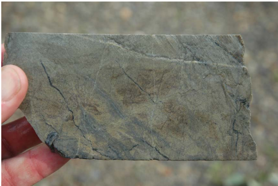
Fig. 4 Remanent patches of potassic (dark) in albite-quartz alteration (light). MK-06-05, 337 m
