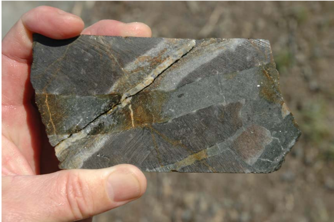
Fig. 5 Veinlets of sericitic (pale gray) cutting albite-quartz alteration (darker gray). MK-09-35, 75-77 m
