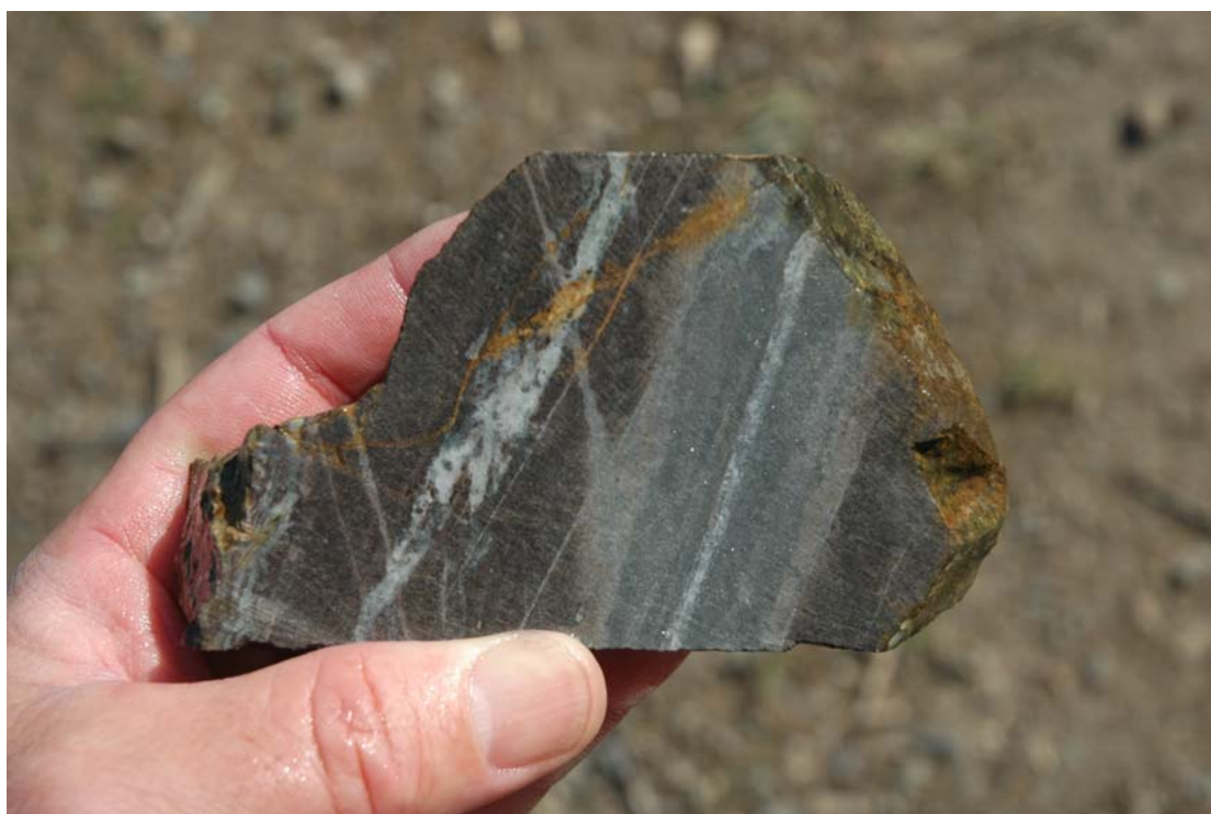
Fig. 6 Quartz-carbonate-sulfide veinlets generated during potassic and overprinted sericitic alteration. MK-09-35, 75-77 m.
