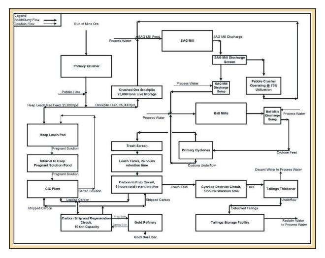
**Figure 16.1** Proposed Livengood process block flow diagram showing both heap leach and mill/CIP process streams.
